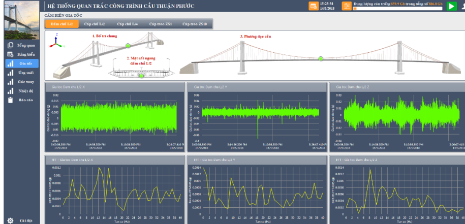
Fig. 19. Panel of accelerometers sensor system
